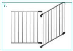
Lift off end section. If gate is now appropriate length, go to step 8.
